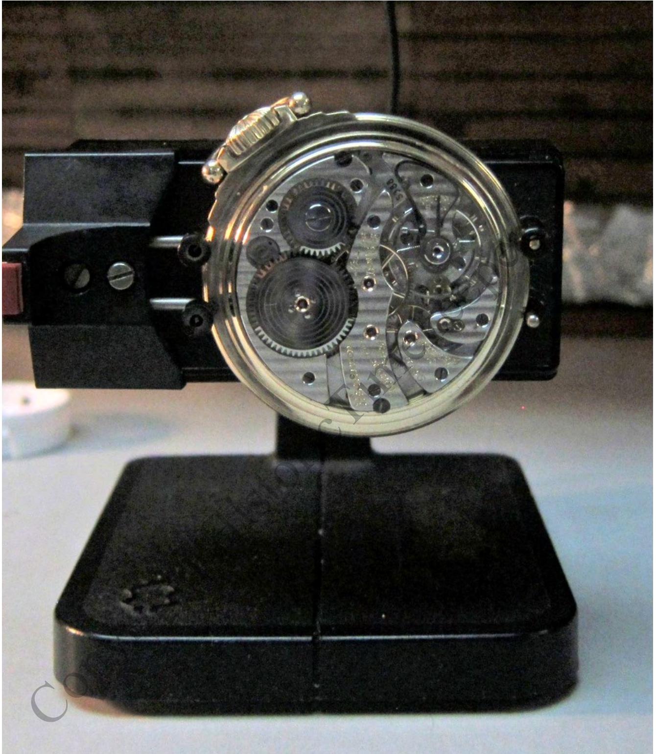
Escape wheel directly below balance
